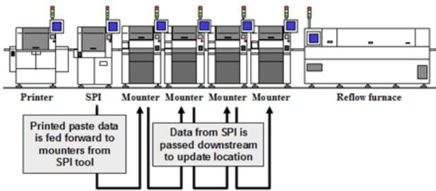
Figure 14: Theoretical SMT Line utilizing Adaptive Process Control
