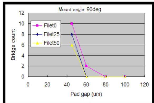
Figure 9: Graphical Results of Solder Bridge Test
