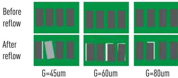
Figure 10 Image of Solder Bridge Test Results
