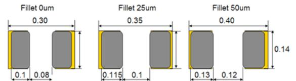
Figure 8: Substrate Pad and Stencil Screen Apertures Conditions
