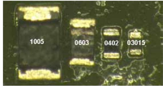
Figure 1: Passive Component Size Comparisons (0402 represents 01005 standard)
